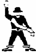
RELEASE SLING LOAD Left arm down away from body. Right arm cuts across left arm in a slashing movement from above
